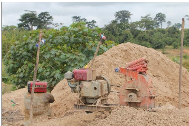
A “Chan fa” machine. A popular hammer mill used by small scale miners. Photo: Lynda Lawson
